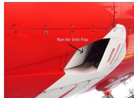
Gambar 4 *Ram air inlet flap*
