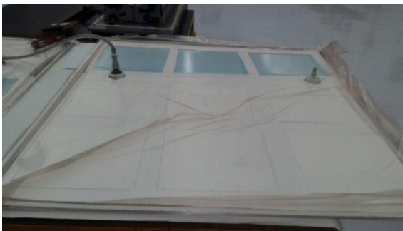
Gambar 3.2 Proses vacuum bagging
