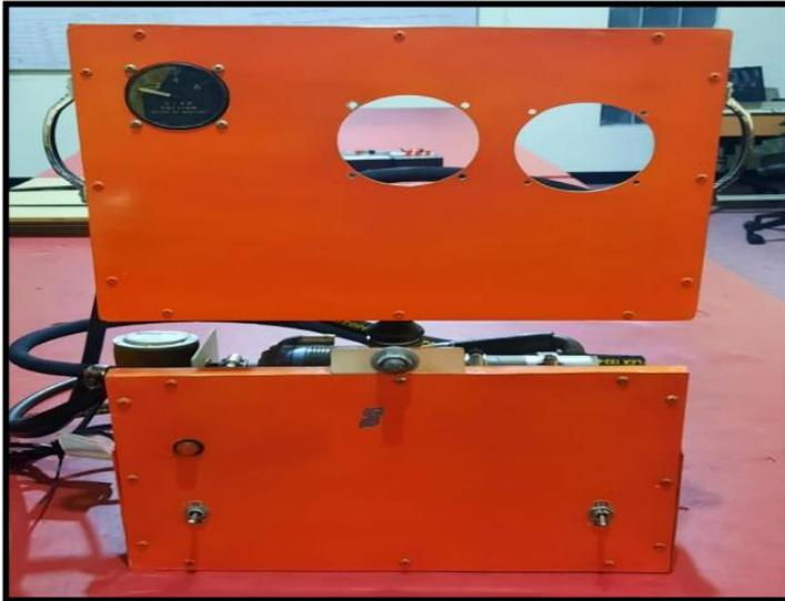
Gambar 5. Tampak depan Alat uji Gyro Horizon Indicator dan Directional Gyro Indicator
