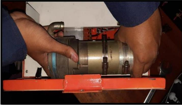
Gambar 3. Pemasangan *Auxiliary Dry Vacuum Pump*
