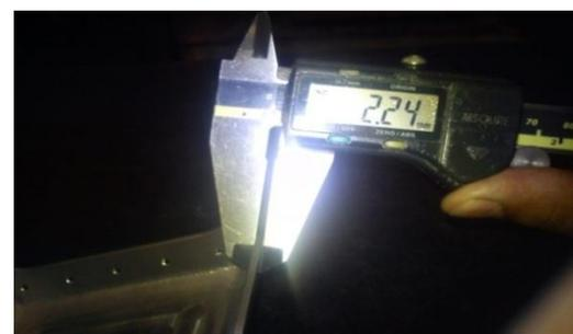
**Gambar 3** out of tolerance
