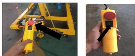
Gambar 3(a) Switch button dan 3 (b) tombol up and down
