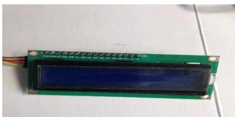
Gambar 2.2 LCD 16x2
