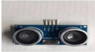
Gambar 2.4 Sensor Jarak HC-SR04
